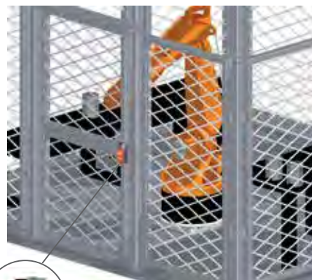
Olympus Solenoid Controlled Access Lock
