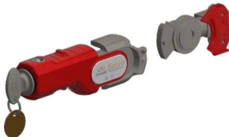
The Salvo Glad Hand Lock (SGL) is a key operated mechanical locking device designed to fit on to all European and US trailer, emergency brake line connectors. Its purpose is to prevent re-connection of the emergency air brake hose, thereby immobilising the trailer. When fitted, the SGL can only be removed with the permit key.
