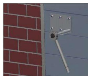
**Step 09:** Drill holes and fix in place using bolts, washers and nuts, supplied. Trim excess bolt length if necessary.
