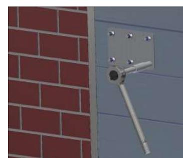
**Step 09:** Drill and pop-rivet two positions. Check that the bolt rotates freely, then drill remaining holes and pop rivet in place.
