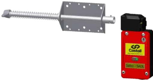
The SADL is a keyless solenoid controlled Lock that locks and unlocks dependent upon the signal received from the Salvo Control Panel (SCP). The unit incorporates a locking bolt which passes through the door running rail and into the lock body. Only when the signal is received from the SCP, can the locking bolt be disengaged, allowing the door to be opened.
