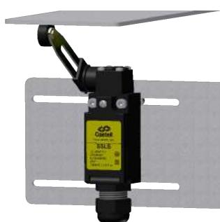
The Salvo Safety Limit Switch comprises a mechanical roller switch and bracket set. It is mounted so that the roller is actuated by the opening and closing of the loading bay door. It should be mounted in accordance with these instructions, in a raised position to prevent accidental damage.
