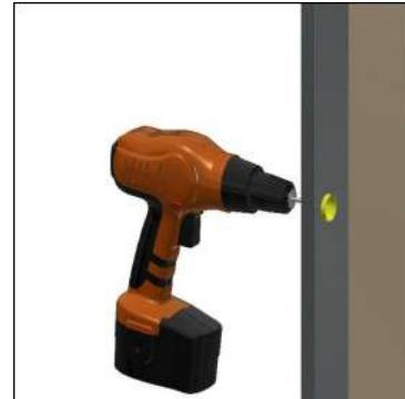
**Step 03:** Drill the clearance hole in the running guide using a 28mm tank cutter.
