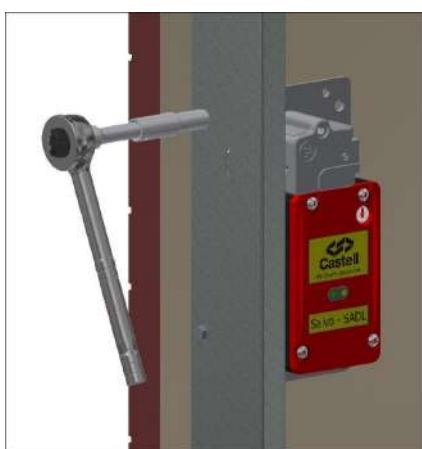
**Step 07:** Fix the lock and bracket in place with the screws provided.
