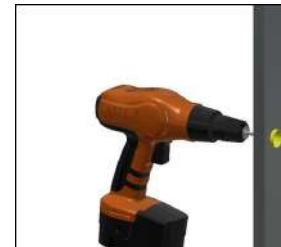
**Step 03:** Drill the clearance hole in the running guide using a 28mm tank cutter.
