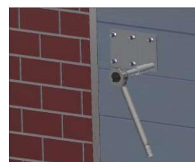
**Step 09:** Drill holes and fix in place using bolts, washers and nuts supplied. Trim excess bolt length if necessary.
