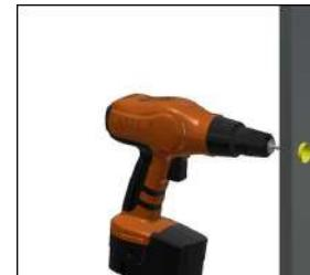
**Step 03:** Drill the clearance hole in the running guide using a 28mm tank cutter.
