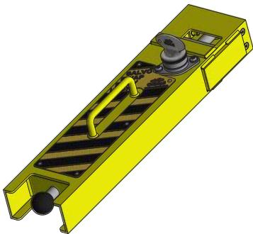
The Salvo Swap Body lock is a key operated mechanical locking device designed to fit into the twist lock aperture on a swap body trailer. When fitted the Salvo Swap Body Lock can only be removed with the permit key. The Salvo Swap Body Lock remains in place when the Castell key is removed. When the loading/ unloading procedures are complete, the Castell key may be inserted, and the Salvo Swap Body Lock removed, allowing the trailer to connect and the vehicle to depart from the loading bay.
