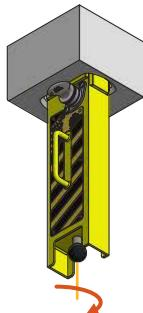
③ Rotate the key anti-clockwise and remove the key. Locking the Swap Body Lock in position.
