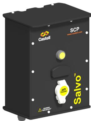
The Salvo Control Panel (SCP) is the main interface between the Salvo couplings and associated bay door controls. The SCP comprises of a wall mounted panel with easy to use Castell interlock key switch to allow operation of the bay. There is also panel indication of status and operation. Installation is via plug in terminals on the internally mounted PCB.
