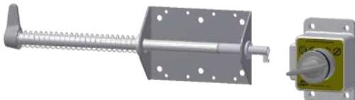
The SMDL-AI (Salvo Manual Door Lock) is a mechanical interlock used to positively bolt loading bay doors in the closed position. The unit incorporates a locking bolt which Passes through the door running rail and into the lock body. Only when the key is inserted and turned, can the locking bolt be disengaged, allowing the door to be opened.
